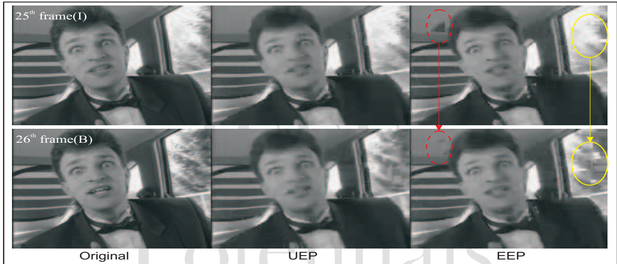
Fig. 7. Carphone sequence transmitted over a noisy channel. The effect of dropped frames due to buffer overflow and the decoder concealment of transmission errors are shown in pictures in the middle and on the right. Source encoder is scalable extension of H.264 which is based on block based DCT. I: Intra frame, B: Bipedicted frame (a frame predicted using two other frames in the sequence), UEP: Unequal error protection, EEP: Equal Error protection.
