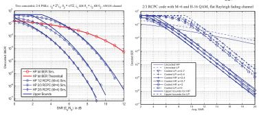
Figure: Simulation results under AWGN and Flat Rayleigh channels.
