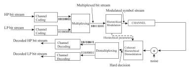
Figure: System block diagram for 2-layer transmission. HP: High Priority, LP: Low Priority.
